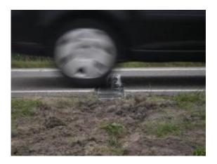
A pilot research project into vibration energy on the N34 provincial motorway near Hardenberg in the eastern Netherlands has shown that vibration energy as a local energy source is a sustainable alternative for the batteries of roadside sensors and other applications. The trial project has provided valuable insights into this innovative form of energy production.
