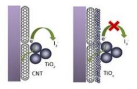
Carbon nanotube electrodes. The use of carbon nanotubes has a significant cost advantage. However, in earlier designs (left), the carbon nanotubes degraded through chemical processes (e-: electrons, I3-: ions in the liquid). Using a thin protective layer of titanium oxide now stabilizes the nanotubes (right), increasing the performance of these cells. Credit: 2011 AIP
