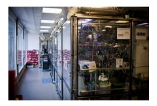
Researchers at the Novartis-MIT Center for Continuous Manufacturing built this drug-manufacturing prototype in an MIT chemical engineering lab. The system, which consists of six connected units, can transform raw ingredients into finished drug tablets. *Photo: Dominick Reuter*
