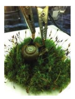
A snail with implanted electrodes connected with crocodile clips to external circuitry. Image credit: L. Halamkova, et al. ©2012 American Chemical Society
