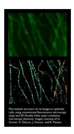
This shows microtubule structure of rat kangaroo epithelial cells with conventional fluorescence microscopy, top, and 3-D Double Helix superresolution microscopy. Credit: G. Grover, K. DeLuca, J. DeLuca and R. Piestun
