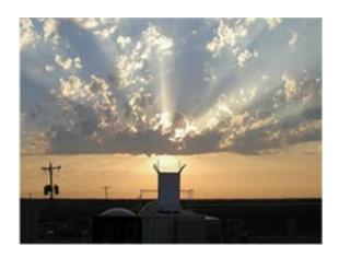
Clouds get in the way of the dawn light, perfectly framing the Raman lidar instrument at the ARM Climate Research Facility Southern Great Plains site. This ground-based laser is a remote sensing instrument used for measuring vertical profiles of several cloud and atmospheric properties.
