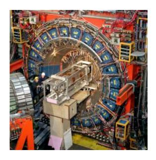
The three-story, 6,000-ton CDF detector takes snapshots of the particles that emerge when protons and antiprotons collide.
