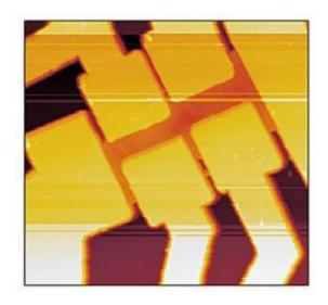
An image of a suspended graphene device made by a scanning probe microscope. The graphene sheet is the orange-colored layer suspended between six rectangular columns made of silicon dioxide and capped by gold. Credit: A.K.M. Newaz, Bolotin Lab / Vanderbilt
