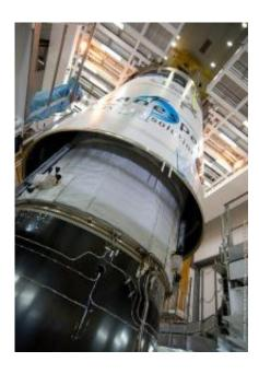
The protective fairing is lowered over Automated Transfer Vehicle Edoardo Amaldi. With the fairing in place, the spacecraft will be lowered on to the Ariane rocket that will launch it to the International Space Station. ESA's third automated space freighter, Edoardo Amaldi, will carry about two tonnes of dry cargo, 285 kg of water and more than three tonnes of propellants to the International Space Station. Credits: ESA/CNES/Arianespace/Optique Video du CSG - J.M. Guillon
