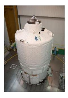
A final view of Automated Transfer Vehicle Edoardo Amaldi before it is installed on the Ariane rocket. ESA's third automated space freighter, Edoardo Amaldi, will carry about two tonnes of dry cargo, 285 kg of water and more than three tonnes of propellants to the International Space Station. Credits: ESA/CNES/Arianespace/Optique Video du CSG - J.M. Guillon
