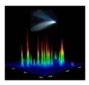
Chromatogram of the cometary ice obtained using the multidimensional gas chromatograph. Each peak corresponds to an amino acid. The higher the peak, the greater is the amount of amino acid present in the sample. *ChemPlusChem*, 77 (2012). Credit: Wiley-VCH GmbH & Co
