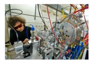
Daniele Filippetto, responsible for APEX's photocathode laser and beam diagnostics, adjusts the mirror that directs the laser to fire into the gun, parallel to the emerging electron beam, to stimulate electron emission from the photocathode. Credit: Lawrence Berkeley National Laboratory photo by Roy Kaltschmidt
