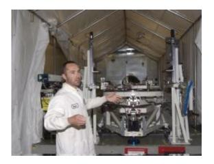
Patrick Johnson, the Webb telescope Optical Test Supervisor at L-3 Tinsley is standing in front of an optical test station used to measure mirror surfaces. Credit: L-3/Tinsley
