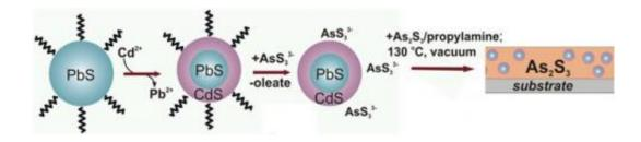
Synthesis of all-inorganic infrared-emitting PbS/CdS nanocrystals and integration into infrared-transparent As2S3 chalcogenide glass matrix
