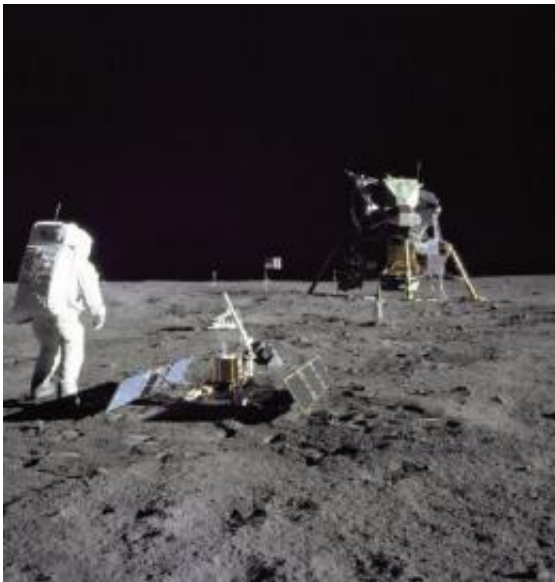
This is Buzz Aldrin placing a seismometer on the moon during the Apollo 11 mission. Credit: NASA
