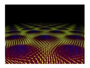
Magnetic eddies in silicon manganese, so-called skyrmions, form a regular grid. Moving these skyrmions needs 100,000 times smaller currents than existing technologies. Credit: Image: TUM
