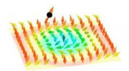
An electron is flying over a grid of magnetic eddies. The forces involved make it possible to control the magnetic structure with a very small current. Credit: Animation: University of Cologne
