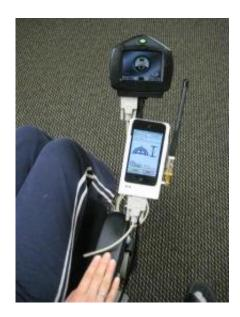
Georgia Tech researchers designed this universal interface for the intraoral Tongue Drive System that attaches directly to a standard electric wheelchair. The interface boasts multiple functions: It not only holds the iPod, but also wirelessly receives the sensor data and delivers it to the iPod, connects the iPod to the wheelchair, charges the iPod, and includes a container where the dental retainer can be placed at night for charging. Credit: Georgia Tech/Maysam Ghovanloo
