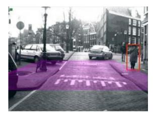
A real of example of how the system detects a pedestrian (red) within a detection area (purple). Credit: C. G. Keller et al.
