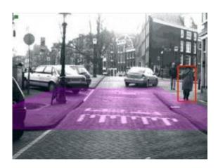
A real of example of how the system detects a pedestrian (red) within a detection area (purple). Credit: C. G. Keller et al.
