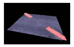
This is a single-atom transistor: 3D perspective scanning tunnelling microscope image of a hydrogenated silicon surface. Phosphorus will incorporate in the red shaded regions selectively desorbed with a STM tip to form electrical leads for a single phosphorus atom patterned precisely in the center. Credit: ARC Centre for Quantum Computation and Communication, at UNSW.
