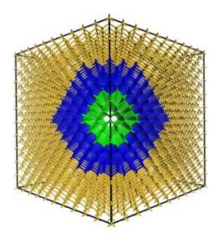
The structure of a small-diameter (green) and large-diameter (blue) silicon nanowire, inside a bulk silicon (yellow) structure. Credit: A\*STAR
