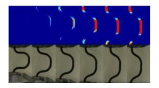
Georgia Tech researchers used a thermal camera to record the variation in surface temperature (top) of a shape-memory alloy experiencing loading and unloading. By inputting this information into their thermo-mechanical model, the researchers were able to accurately predict internal temperature and stress distributions for the material, which is being investigated for use in constructing seismic-resistant structures. Credit: Georgia Tech/Reza Mirzaeifar
