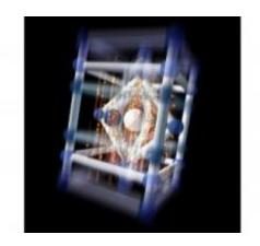
This artist's conception depicts the sudden contraction and elongation experienced by the unit cell of the ferroelectric material lead titanate as an intense pulse of violet light hits it. This atomic-scale wiggle represents the first step in the photovoltaic response that light produces in this and related materials. Illustration by Gregory M. Stewart/SLAC National Accelerator Laboratory
