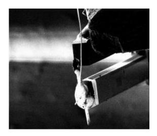
For their experiments the IBM scientists used their home-built combined scanning tunneling microscope (STM) and atomic force microscope (AFM). In this focused ion beam micrograph, the tip attached to a tuning fork can be seen. The tuning fork measures a few millimeters in length. The tiny tip measures only a single atom or molecule at its apex.
