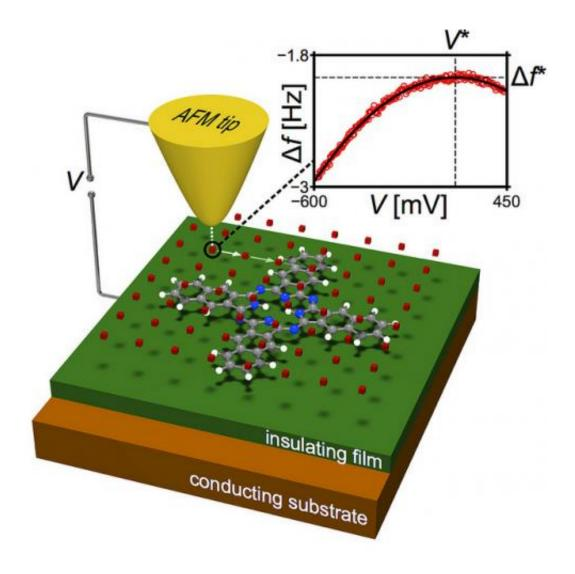
Schematic of the measurement principle. At each tip position, the frequency shift is recorded as a function of the sample bias voltage (inset, red circles). The maximum of the fitted parabola (inset, solid black line) yields the KPFM signal V\* for that position. Image courtesy of IBM Research - Zurich
