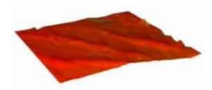
The three-dimensional features of a snow field above treeline is revealed by laser measurements. The laser, installed by NCAR at a test site in the Rocky Mountains, measures snow at more than 1,000 points across an area almost the size of a football field. Credit: ©UCAR, Image by Ethan Gutmann, NCAR
