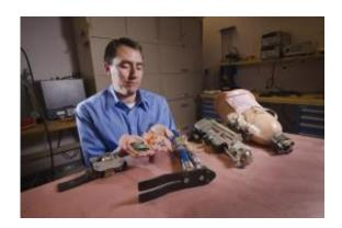
Robotics engineer Steve Buerger displays implantable and wearable neural interface electronics developed by Sandia as he sits in the prosthetics lab with a display of prosthetic components. He is part of a research team that is working on ways to improve amputees' control over prosthetics with direct help from their own nervous system. Credit: Randy Montoya
