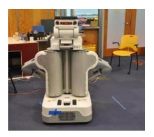
The researchers used at PR2 robot, developed by Willow Garage, with a Microsoft's Kinect sensor to test their system. Image: Hordur Johannsson
