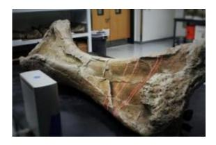
A laser scanner creates a 3-D digital scan of the fossil humerus from *Paralititan*, one of the largest sauropod dinosaurs ever found. Using a 3-D printer, the shape of the scanned fossil can be built at a smaller scale for modeling and testing the mechanics of movement. Credit: Drexel University
