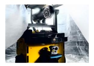
Equipped with multiple sensors and optical cameras, the mobile robot roams over dangerous ground. Credit: Fraunhofer IOSB
