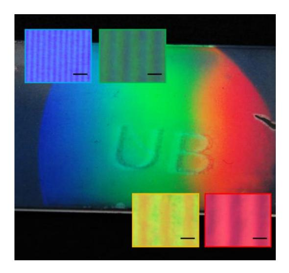
This is a rainbow-colored grating, about 25 millimeters wide, under sunlight. Enlarged microscope images show the graded surface, with the black bars indicating a length of 10 microns. Credit: University at Buffalo
