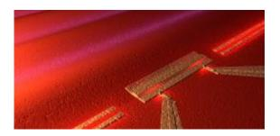
A "quantum microphone" based on a Single Electron Transistor (SET) detects sound waves on a chip surface, so called Surface Acoustic Waves (SAW). The waves make the charge of the atoms underneath the quantum microphon oscillate. Since the quantum microphone is an extremely sensitive charge detector, very low sound levels can be detected. (The size of the waves are exaggerated in the picture). Picture: Philip Krantz, Chalmers
