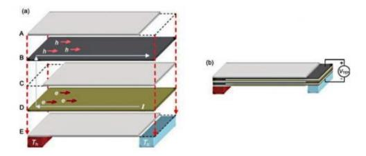
When the multi-layer fabric is exposed to a temperature gradient, charge carriers (electrons or holes) travel from the hot side to the cold side due to the Seebeck effect. The resulting voltage can be read across the ends of the first and last conduction layers. Image credit: Hewitt, et al. ©2012 American Chemical Society
