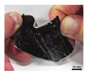
The flexible, lightweight CNT/polymer thermoelectric fabric contains hundreds of alternating layers of conducting and insulating material. Image credit: Hewitt, et al. ©2012 American Chemical Society
