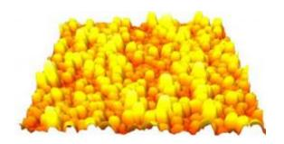
Figure 1: The polymer film forms nanodots: tiny bumps that can be functionalized with antibodies to grab passing cancer cells. Credit: Reproduced, with permission, from Ref. 1 © 2011 WILEY-VHC Verlag GmbH & Co.
