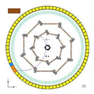
A view of one of the three events found by FINUDA: a schematic frontal view of the apparatus is shown, and the two blue lines represent the two 'pi' mesons moving along opposite bent trajectories in the magnetic field of the apparatus. Image credit: FINUDA collaboration
