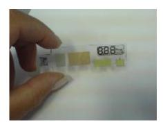
(PhysOrg.com) -- Paper-thin sensors that use the latest technology in miniaturization and printing could revolutionize the way point of care testing is carried out for cholesterol and lead to further applications and developments of the technology.
