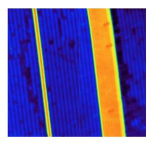
A one-dimensional quantum nanowire (seen in yellow on left) can turn from a conductor to an insulator with the addition of a single atomic defect, according to microscopic analysis from Oak Ridge National Laboratory. Bundles of nanowires (right) are generally more stable, leading to better conductance. Credit: An-Ping Li and Shengyong Qin/ORNL
