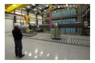
Gary Bass, from the Naval Surface Warfare Center in Dahlgren, Va., uses a crane to maneuver a 32-MJ version of the Office of Naval Research-funded Electromagnetic Railgun prototype into place for government evaluation. The EMRG is a long-range weapon that launches projectiles using electricity instead of chemical propellants and is under development by the Department of the Navy for use aboard ships. Credit: US Navy photo by John F. Williams/Released
