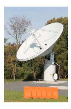
This 12-meter radio antenna is a new addition to a faster and more sensitive VLBI (Very Long Baseline Interferometry) system being developed at the Goddard Geophysical and Astronomical Observatory. The goal for the new system is to be able to measure down to the millimeter, or about the thickness of a penny. Credit: NASA/GSFC/Elizabeth Zubritsky
