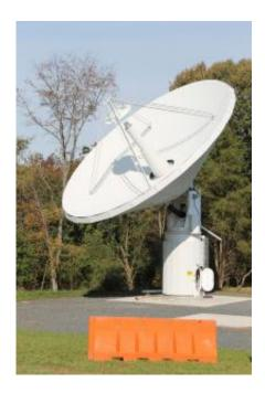
This 12-meter radio antenna is a new addition to a faster and more sensitive VLBI (Very Long Baseline Interferometry) system being developed at the Goddard Geophysical and Astronomical Observatory. The goal for the new system is to be able to measure down to the millimeter, or about the thickness of a penny. Credit: NASA/GSFC/Elizabeth Zubritsky
