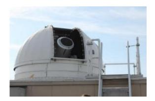
The telescope on NASA Goddard's Next Generation Satellite Laser Ranging (NGSLR) system peeks through the open dome. The NGSLR laser ranges to Earth-orbiting satellites and to NASA's Lunar Reconnaissance Orbiter. Credit: Credit: NASA/GSFC/Elizabeth Zubritsky
