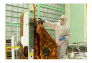
Aleksandra Bogunovic reaches across the instrument to affix the corners of a Multi-Layer Insulation blanket to the TIRS instrument. The Thermal Infrared Sensor (TIRS) will fly on the next Landsat satellite, the Landsat Data Continuity Mission (LDCM). TIRS was built on an accelerated schedule at NASA's Goddard Space Flight Center, Greenbelt, Md., and will now be integrated into the LDCM spacecraft at Orbital Science Corp. in Gilbert, Ariz. Credit: NASA Goddard/Rebecca Roth
