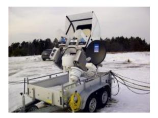
The University of Bonn ADMIRARI Radiometer deployed at the CARE site. This instrument measures microwaves that are naturally emitted from Earth's surface to determine water vapor and cloud and liquid water in the air column. Credit: NASA / Walt Petersen
