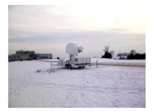
The NASA D3R radar deployed at the CARE site. This radar scans the air column for snow falling from the clouds to the ground. Credit: NASA / Walt Petersen
