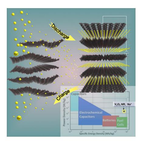
The electrostatic attraction of electrochemically altered V2O5 layers provides a strong driving force for Na+.
