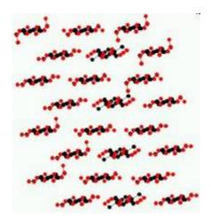
Chain model of the cellulose molecules, as examined using neutron scattering at the ILL.
