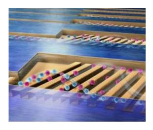
A new microfluidic device isolates target cells (in pink) from the rest of the flow by getting them to stick weakly to the device's ridges, then roll through trenches, and into a collection chamber. Image: Nicolle Rager Fuller
