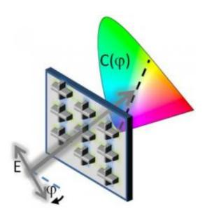
The color output of a new type of optical filter created at Harvard depends on the polarization of the incoming light. Credit: Image courtesy of Tal Ellenbogen.
