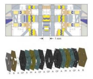
A small portion of the CAD design for the Harvard Monolithic Bee illustrates the complexity of folds and joints necessary for its assembly. Using the old, manual process, every one of those parts would have to be cut, folded, assembled, and glued by hand. The bottom image illustrates the 18 layers of lasercut materials that create the pop-up structure. Credit: Images courtesy of Pratheev Sreetharan, Harvard School of Engineering and Applied Sciences.
