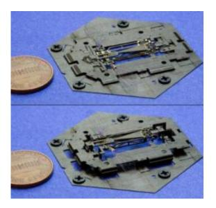
The Harvard Monolithic Bee (or "Mobee") pops up within an assembly scaffold, which performs more than 20 origami assembly folds. Credit: Photos courtesy of Pratheev Sreetharan, Harvard School of Engineering and Applied Sciences.
