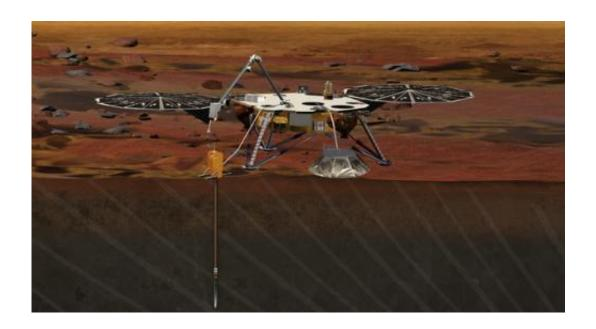
Artist rendition of the proposed InSight (Interior exploration using Seismic Investigations, Geodesy and Heat Transport) Lander. InSight is based on the proven Phoenix Mars spacecraft and lander design with state-of-the-art avionics from the Mars Reconnaissance Orbiter and Gravity Recovery and Interior Laboratory missions. Image credit: JPL/NASA
