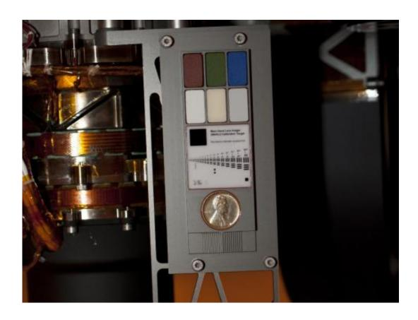
NASA's Mars rover Curiosity with an inset showing calibration targets to be used by a camera at the end of the robotic arm. Image credit: NASA/JPL-Caltech
