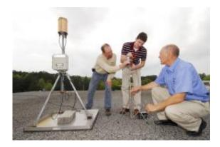
John Trostel, Matthew Bond and Tom Perry adjust a student-designed field mill operating on the roof of GTRI's Cobb County Research Facility. To the left is a commercially made field mill. Credit: Gary Meek
