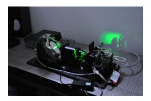
ABSL prototype lidar, intended to help a lander touch down safely on a planet, detecting and avoiding hazards Credits: ESA/ABSL
