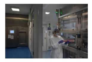
Automation and manual operation have to go hand in hand in tomorrow's laboratories: a rack with reagents is checked prior to the insertion in an automated cell cultivation system. Credit: Fraunhofer IBMT
