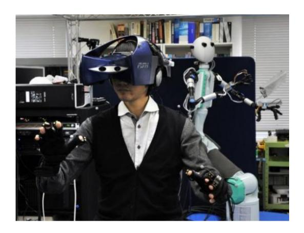
An operator -- wearing a special HMD and a pair of gloves -- controls the "Telesar V" (right) that was developed by Keio University's Graduate School professor Susumu Tachi (not in the picture) at his laboratory in Yokohama, suburban Tokyo. The robot that mimics the movements of its human controller is bringing the Hollywood blockbuster "Avatar" one step closer to reality.
