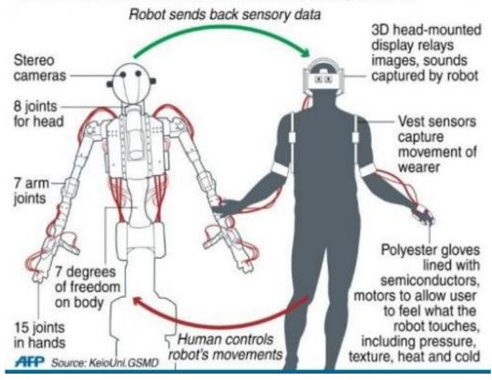
Graphic on the TELESAR V robot that mimics the movements of its human controller, and relays back data on what it sees, hears and feels
