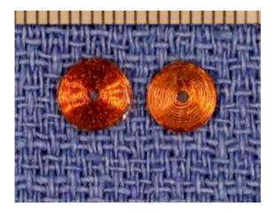
(PhysOrg.com) -- A new implantable sensor developed at Rensselaer Polytechnic Institute can wirelessly transmit data from the site of a recent orthopedic surgery. Inexpensive to make and highly reliable, this new sensor holds the promise of more accurate, more cost-effective, and less invasive post-surgery monitoring and diagnosis.
